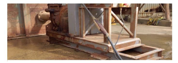
Slurry pumps are mostly large in size and notoriously difficult when it comes to undertaking maintenance and repair. It is a task that usually requires more than one person, the use of lifting aids and one that poses the danger of possible injury to those undertaking the operation.
